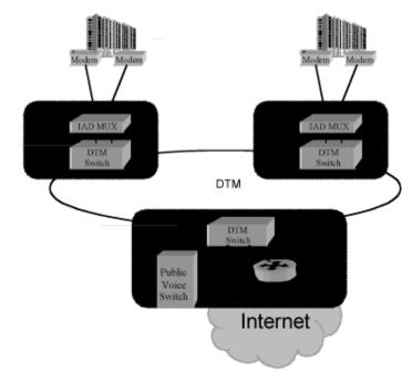
Figure 10: DTM Network for Integrated-Access–Device Aggregation
