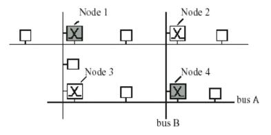
Figure 5: Switch node interconnection
