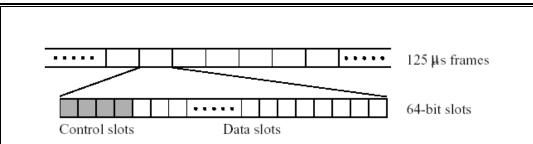
Figure3: DTM Multiplexing Format
