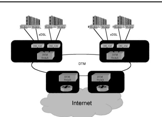
Figure9: DSLAM Aggregation Network for Internet Connections
