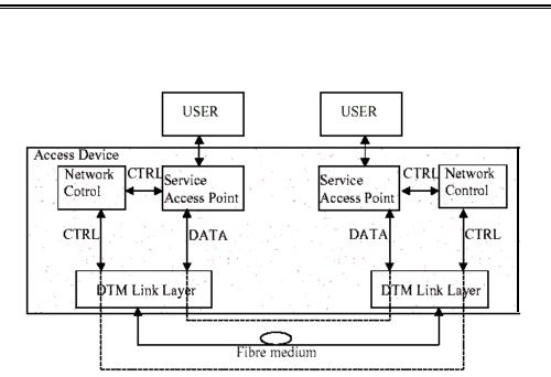
Figure4: Flow of data and control information
