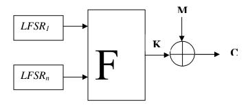
In this model, Fig-1. Stream Cipher System
