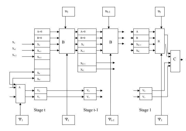
Pipeline Architecture A: Initial circuit B: Intermediate circuit C: Final circuit.
